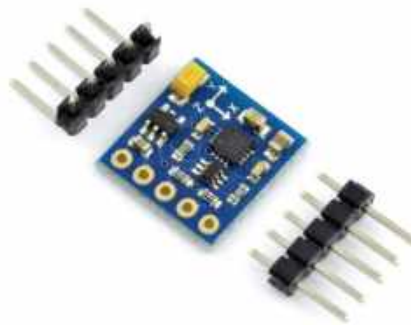
Rys. 7. Magnetometr GY-271, HMC5883L [6]
